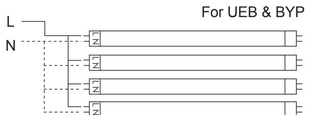
Step 2. For non-shunted holders, wire the holders and lamps according to the diagram.
