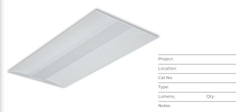
The Philips Day-Brite / Philips CFI Recessed FluxGrid LED offers architectural appeal with "must have" features. Two different lens styles, discrete air handling, integral emergency, and access to the boards and driver from below make FluxGrid an ideal solution for a wide range of applications.
