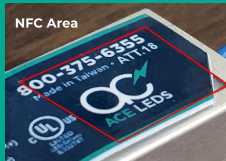
3. Place the NFCPRO3 Programmer directly on top of the NFC area of the driver and press the green **“OK”** button. If successful, the device will beep once and will display a red **“PASS”**. Otherwise, it will beep 3 times and display a red **“FAIL”**.
