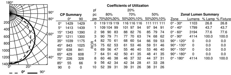
**BLT4 48L ADP LP835**, 4888 delivered lumens, test no. ISF35685P114, tested in accordance to IESNA LM-79
