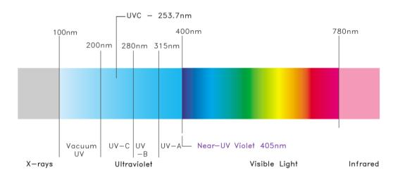
UV-C - germicidal ultraviolet light - is a proven technology to effectively disinfect air and surface 253.7nm refers to the most effective wavelength frequency of the ultraviolet light UV-C can cause health hazard to the skin and eyes if improperly installed and used
