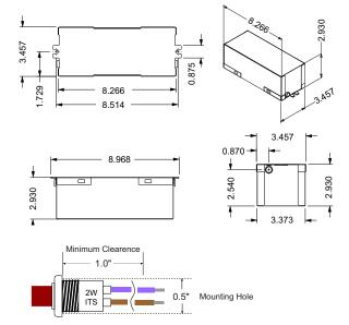
An illuminated test switch/charging indicator light is provided.
