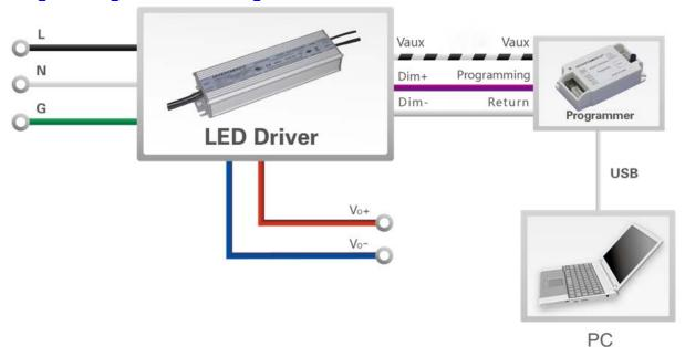
**Note:** The driver does not need to be powered on during the programming process.
