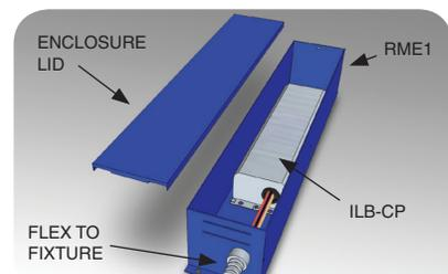
The RME1 enclosure accepts "B" configuration ILB-CP units for remote mounting. The ILB-CP is secured within the enclosure and wiring is routed through the 2 ft. of flexible conduit for connecting to the fixture. Can be used in conjunction with the TBMK for grid ceiling mounting.
