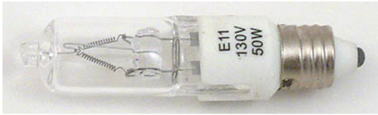
50 Watt E11 (Miniature Candelabra) Base, 130 Volts, Clear, 2.17 Inches Long
