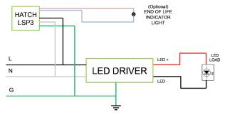
**EOL Indicator:** When illuminated, LSP3 is working correctly. When the indicator goes out, LSP3 needs to be replaced as soon as possible.
