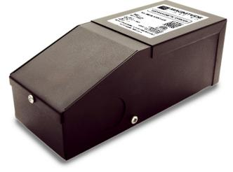
Magnitude's M50L12DC-AR is the most compact LED driver on the market with a magnetic transformer core. It is equipped with two auto-reset breakers, one on the input and one on the output, which protect both the load and driver. The driver is encased in a coated metal box that includes 2 knock-outs, one on each side, to enable easy installation that complies with electrical code requirements.
