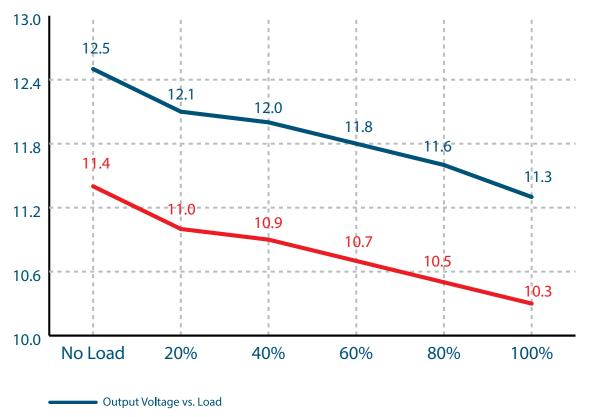
Output Voltage With a Typical Dimmer
