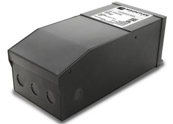
Magnitude's T180L12DC is a multi-output class 2 LED dimmable LED driver. It is equipped with push-to-reset breakers, one on each output, protecting both the load and the driver. Encased in a high-quality NEMA 3R metal case enclosure, that includes 5 knock-outs to enable easy installation. All of our T- Series LED Drivers are dimmable with any standard MLV TRIAC dimmer.
