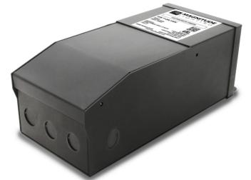
Magnitude's T192L24DC is a multi-output class 2 LED dimmable LED driver. It is equipped with push-to-reset breakers, one on each output, protecting both the load and the driver. Encased in a high-quality NEMA 3R metal case enclosure, that includes 5 knock-outs to enable easy installation. All of our T- Series LED Drivers are dimmable with any standard MLV TRIAC dimmer.
