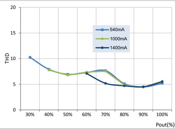
THD vs Output Voltage at 230Vac
